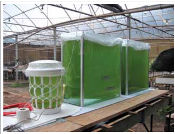
Figure 1. Inoculum and 300 L C. sorokiniana culture kept under semi-controlled conditions. Image: Lombardi AT, Algae Biotechnology Laboratory, Botany Department (UFSCar) (UFSCar)
