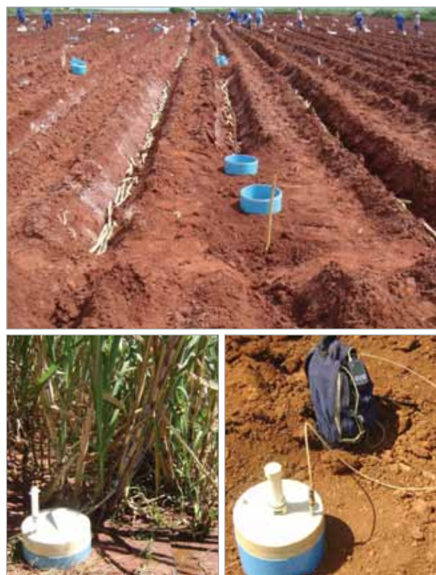
Figure 1. Field experiment with stalk seeds of sugarcane inoculated with diazotrophic bacteria. Blue tubes are the bases of chambers installed to allow the collection of green house gases, including N 2 O, emitted from soil and N fertilizer. Gas sampling in the field
